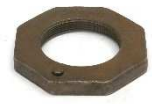
ZE2128 Replacement Service Nut Used in place of ZE1253 to convert to "Manual" adjustment. 3-3/16"OD 2-3/8"ID 1/2" Thick
