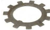
ZE3010 Lock Tab Used with Positive Adjust Nut or replacement service nut to lock outer nut in place. 4"OD 1-13/32"ID
